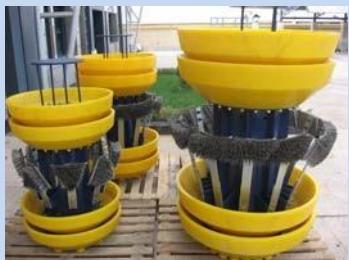
Cleaning pigs are manufactured to remove dust and debris in the pipeline. The standard pig is designed to traverse 1.5 D radius bends to 3D according to the length of the pig. They have a central body equipped with wire brushes to scrap internal part of the pipes. Pigs with 14" or smaller diameter with centre-rod type body normally use
