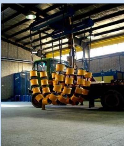
Roller cradles are designed to provide the supports in operation of pipeline lifting machineries. Each of them can carry different sizes of pipes. Various cradle assemblies for pipe sizes 6" through 56" are available with associated replacement rollers. The cradle design provides quick disassembly for transit and storage. Different polyurethane rollers are configured to support the pipe evenly and to prevent any damages on coating.
