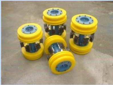
Bi-Directional pigs are manufactured for bi-directional running. They are used for cost effective hydrostatic testing in filling and dewatering operations without removing the pig displacing and batching, line evacuation of air or liquids de-waxing and pre-inspection cleaning. The standard pig is designed to traverse 1.5D radius bends to 3D, according to the length of the pig. Pigs
